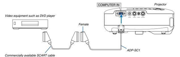
Before connections: An exclusive SCART adapter (ADP-SC1) and a commercially available SCART cable are required for this connection.
